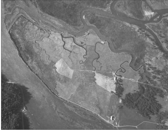
1939 Aerial (note channel connections and lack of ditches)
