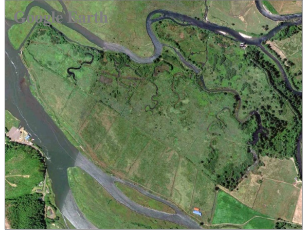
2011 Aerial (note blocked channels and extensive ditching)
